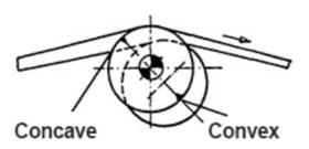
When the middle of the web is slack the convex side of the roller is swung out from its normal position until the middle of the web is tensioned properly.
