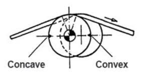
When processing webs with slack edges the concave side of the roller is swung out from its normal position until the edges bear firmly on both ends of the roller.
